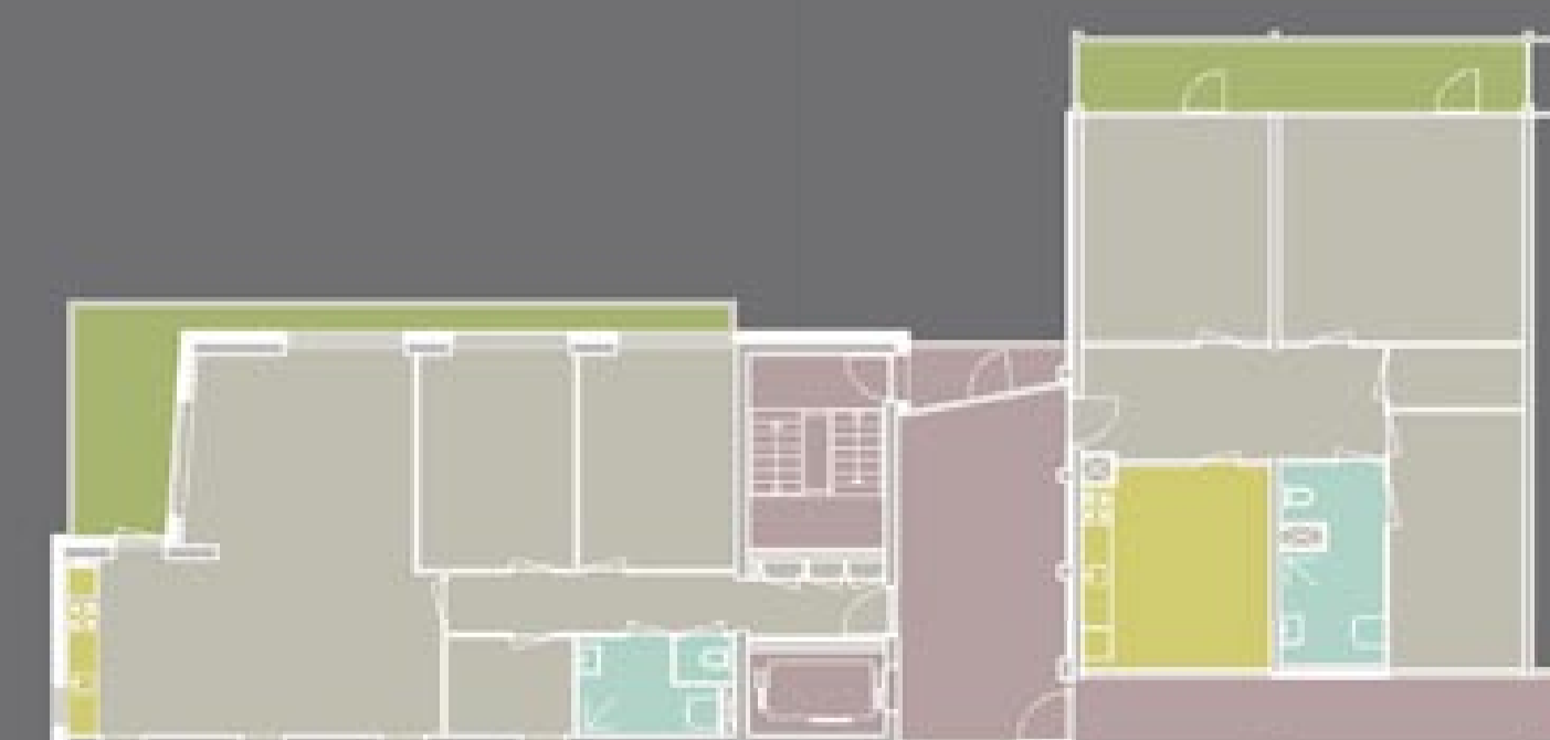
floorplan added highrise on the head; new elevator is connected to existing gallery
