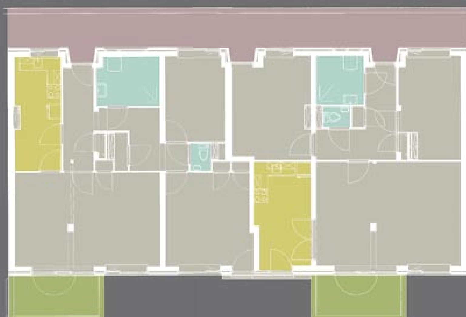
new floorplan 2 nd and 3 rd floor: gallery apartments (elderly) by making three-to-two
